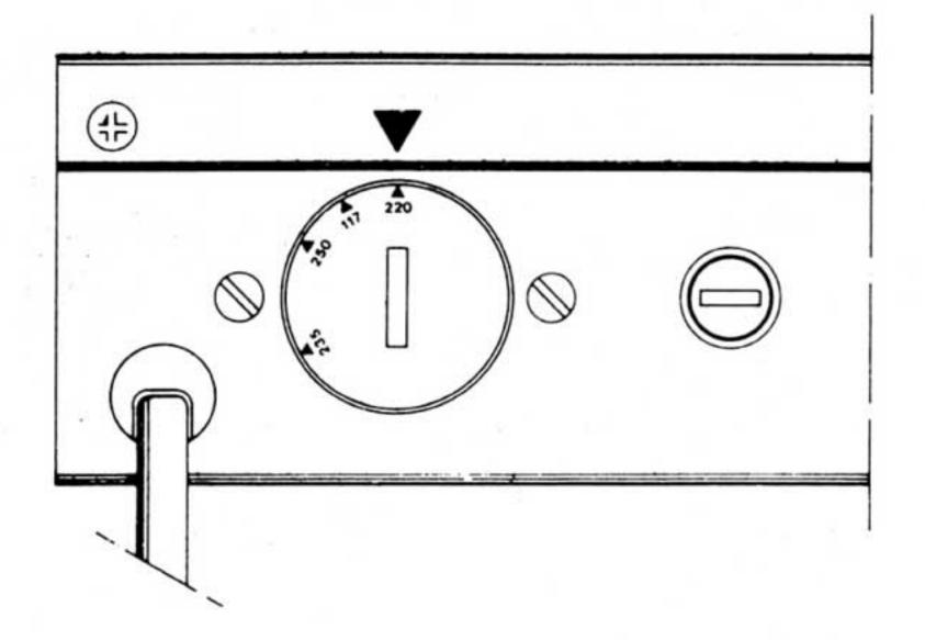
A fuse holder ③ is located next to the voltage selector. The fuse should be 4,0 Amp slow for 117 V power supply, 2,0 Amp slow for other voltages.
