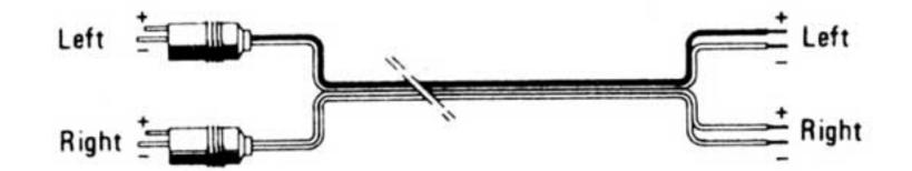
The satellite speakers should be connected in parallel to the two subwoofer channels, either at the amplifier, or at extra terminals on the Subwoofer. Use the most convenient connection method.
