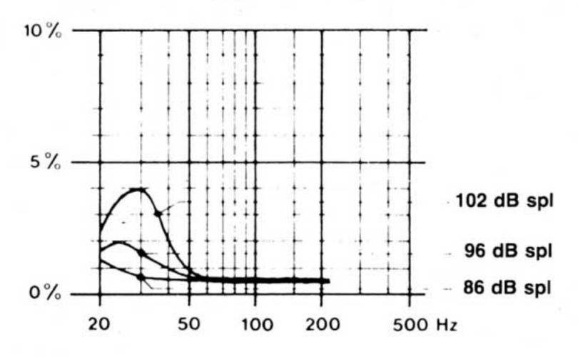
Typical distortion at different output levels. 2nd + 3rd harmonics.
