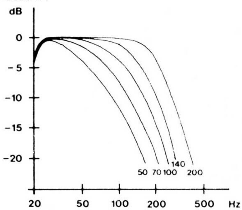
If the Subwoofer is connected to the speaker outputs of the main amplifier (as in 4 B-, and consequently the low bass of the satellite speakers cannot be cut off, the knob should be set to the frequency where the response of the satellites are down 3 dB.
