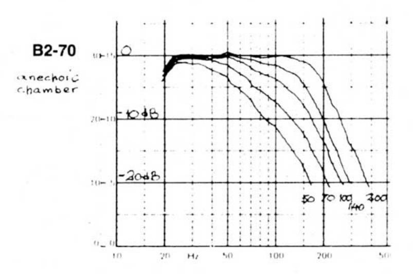
Frequency response at different settings of upper frequency limit.
