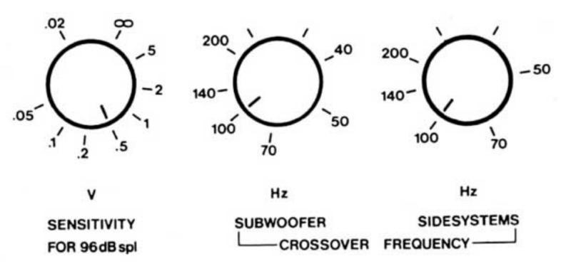
There are three control knobs on the top of the Subwoofer's amplifier cabinet, seen above.
